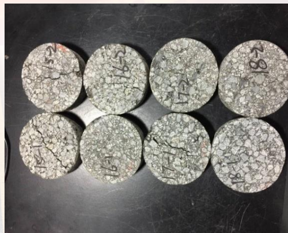
劈裂后芯样 after test
