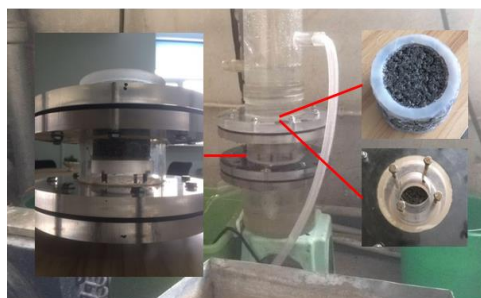
A horizontal permeability test
