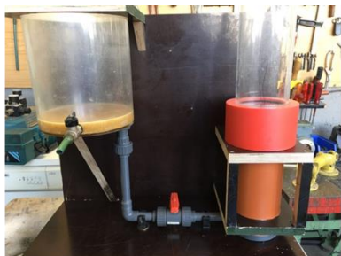
A U-shape Vertical Permeability Test
